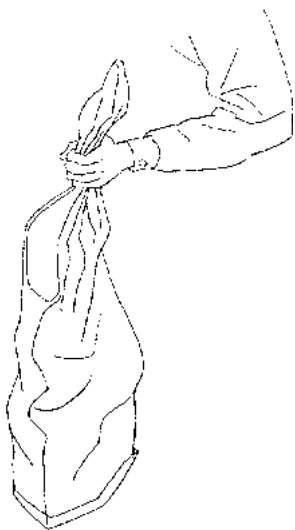
Figure 12A: Sandbag filled 1/4 to 1/3 full
